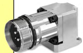
Panel connector, front mount angled, fixed, with axial O-ring square flange, 4 holes 4.2 mm Ø to be phased out **A F 0 0**
